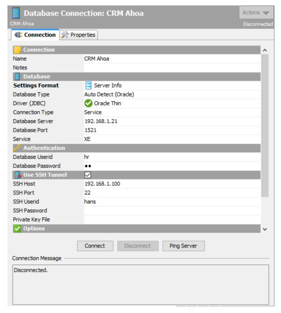
The **SSH Host** is the name or IP address for the host accepting SSH connections. The SSH Host is typically the same as the Database Server. Enter the port for SSH connections in the **SSH Port** field. The default value is 22.
